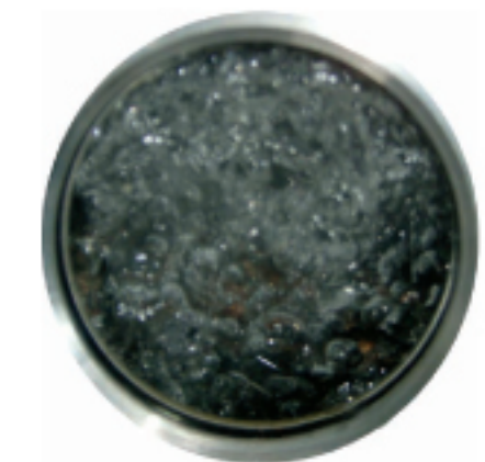
Boiling bubbles from brine @ Evaporator by jacket water heating
